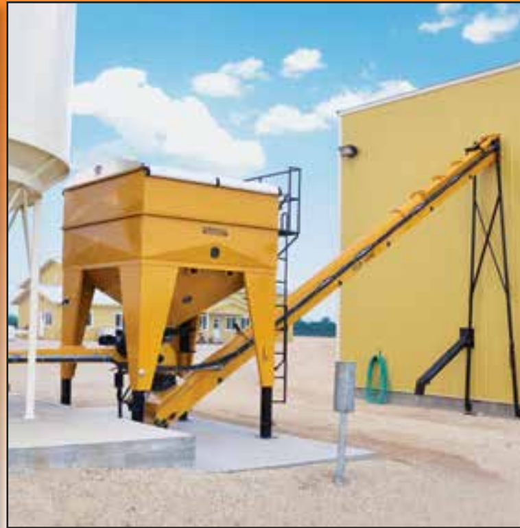
The conveyor can be permanently placed without an undercarriage, to operate on site.
