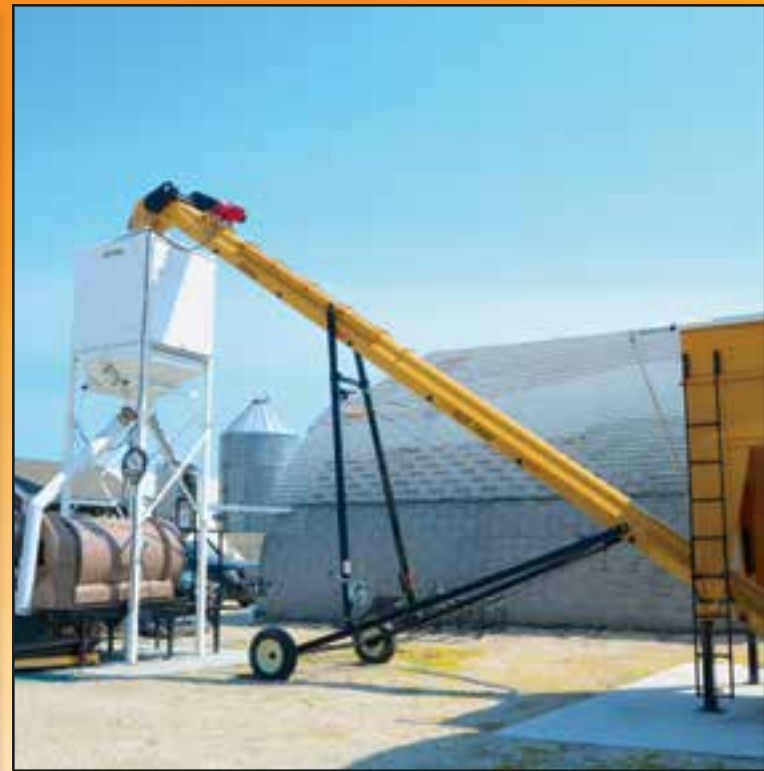
The conveyor can be used in a permanent, self-supporting configuration.
